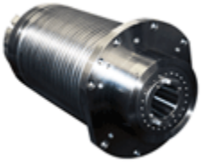
ES750 - H6161H1043 Kw 30-S1/36-S6 - ISO50 - 224Nm S1 - 10.000rpm - liquid cooling 380V - DPC - encoder HSD TTL
