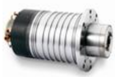
ES796 - H6161H0935 Kw 15,0-S1/18,0-S6 - ISO40 - 12.000rpm - liquid cooling 380V - DPC - encoder LB TTL
