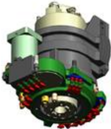
ES796 MK353 - H6314H0647 Kw 15,0-S1/18,0-S6 - ISO40 - 12.000rpm - liquid cooling 380V - body - C Axis - speed ratio 1/200 - DPC - encoder LB TTL
